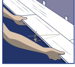
Step 4: Lock long edge of flooring by inserting tongue into groove at an angle and drop in place. Slide flooring toward end of previously installed flooring until the tongue just touches the groove.
