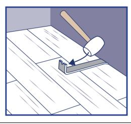
Step 9: Use hammer and pull bar to lock long edges of flooring on final row.
