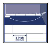
**Step 3:** Use leftover plank from first row as starter for second row. Minimum 8" stagger between plank end joints.
