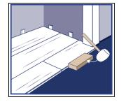
Installation under door jambs: Step 1: Undercut door jamb to allow plank to slide freely. Use a tapping block to lock planks.
