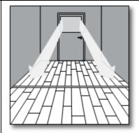
Try to run planks parallel to main light source.
